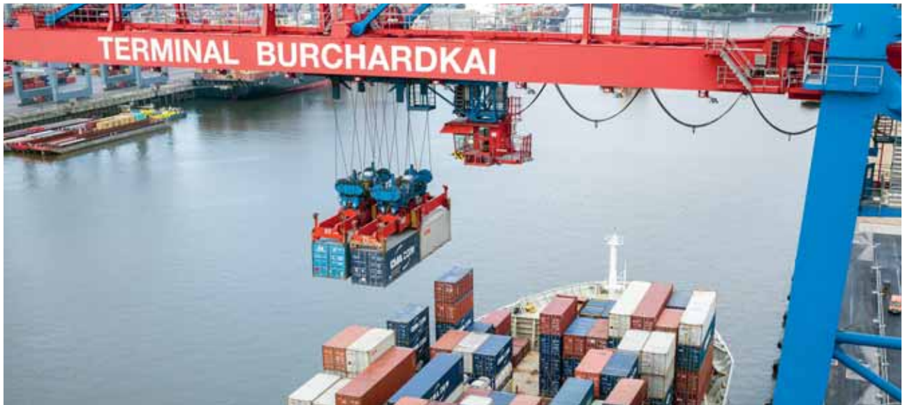
Innovative duo: tandem gantry cranes discharge four 20-foot containers in a single movement.
