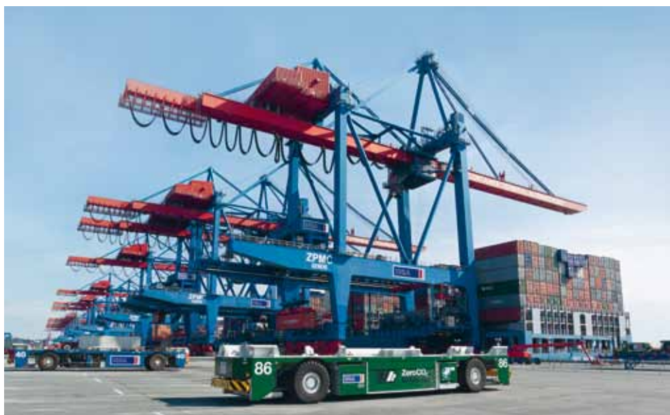
Battery-powered automated container transporters (AGVs) at the HHLA terminal in Hamburg-Altenwerder
