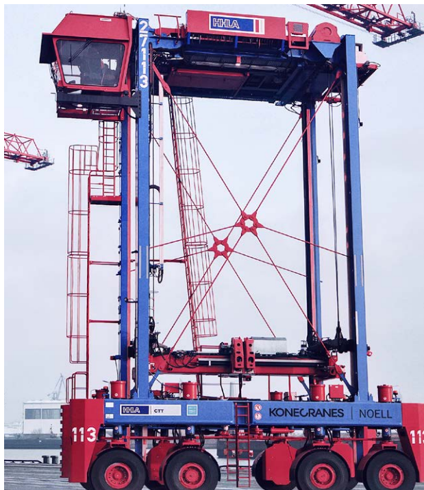
The new hybrid van carriers at the CTT and CTB consume 25% less diesel.
