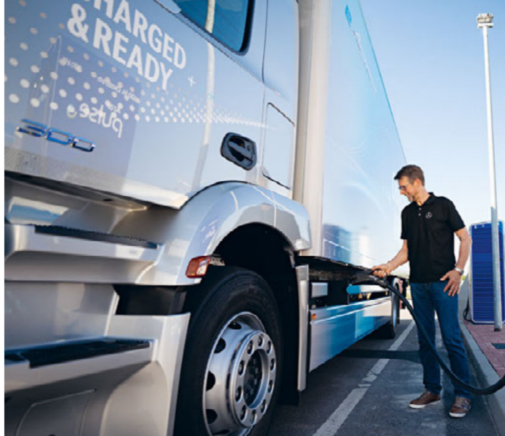
ELECTRIC ROAD TRAFFIC At 300 kilowatts, vehicles can be charged with enough green electricity in 45 minutes to travel around 200 km. The first 600 kilometres of motorway between Dortmund and Schegenheim have been equipped for e-trucks. Many more will be needed in future.
